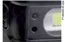
Move your hand in front of the sensor: it turns on and off. No need to touch it
